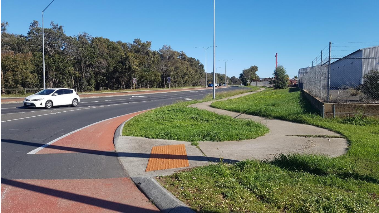
Photo 10: Narrow footpath with non-standard pedestrian ramp. Footpath does not continue on far side of Ozich Court.
