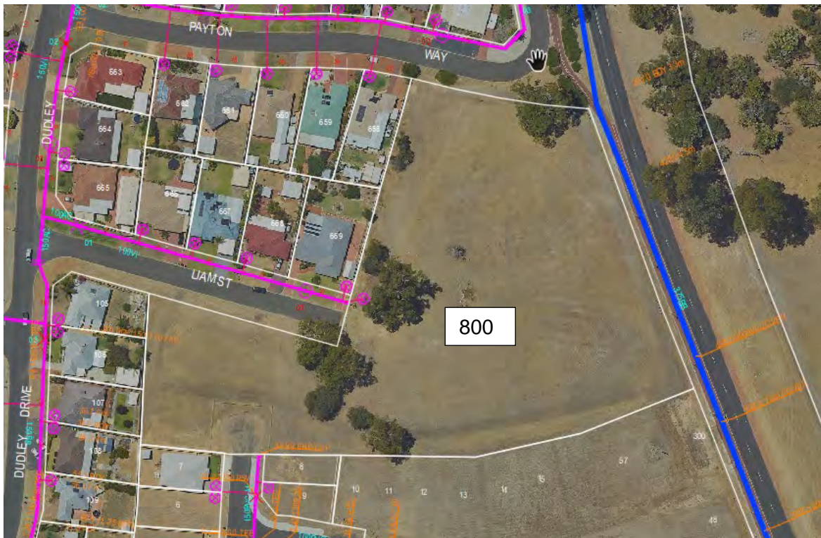
Figure 29 Water mains servicing Lot 800 (Aqwest)
