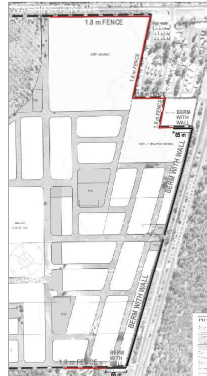
Figure 15 Recommended Noise Attenuation Measures
